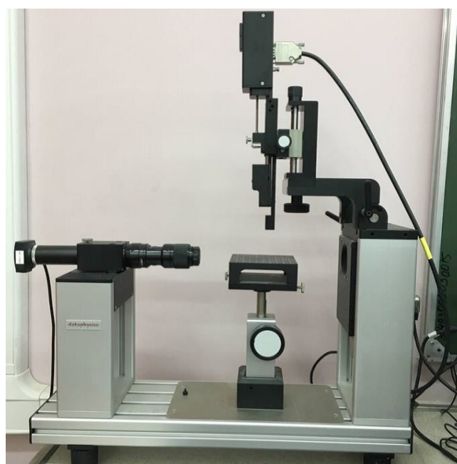
Fig. 2. External view of the Dataphysics OCA 15ES instrument
