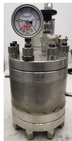
Figure 2. High-pressure cell for hydrate saturation of samples (manufactured together by KryoLab LLC and FabLab & Machine Shop, Russia)
